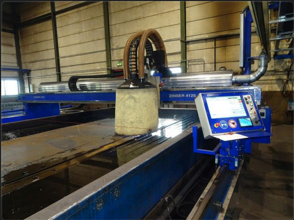
Zinser 4125 Underwater plasma cutting system
